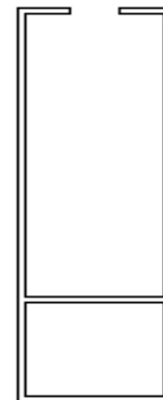
Fig. 28 – Example for a baffle made from extruded aluminium
