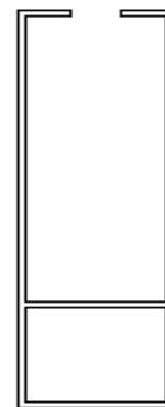
Fig. 27 – Example for a double-walled baffle made from extruded aluminium
