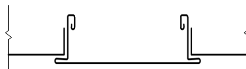
Fig. 10 – Example for a lay-on post-cap system
