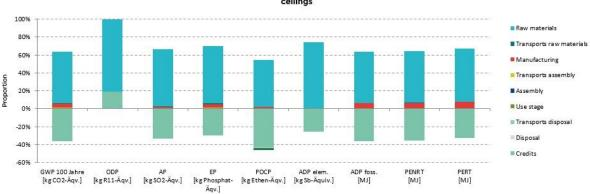
Relative contributions of the stages of the life cycle of 1 kg metal ceiling systems made of steel as cooling and heating ceilings
